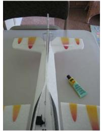
Next are the aileron controls rods (CF and heatshrink type shown). Detail pic of control horn shown below.
