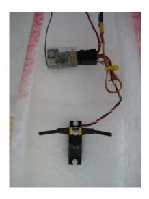
The rudder servo should be the same height as the control horn
